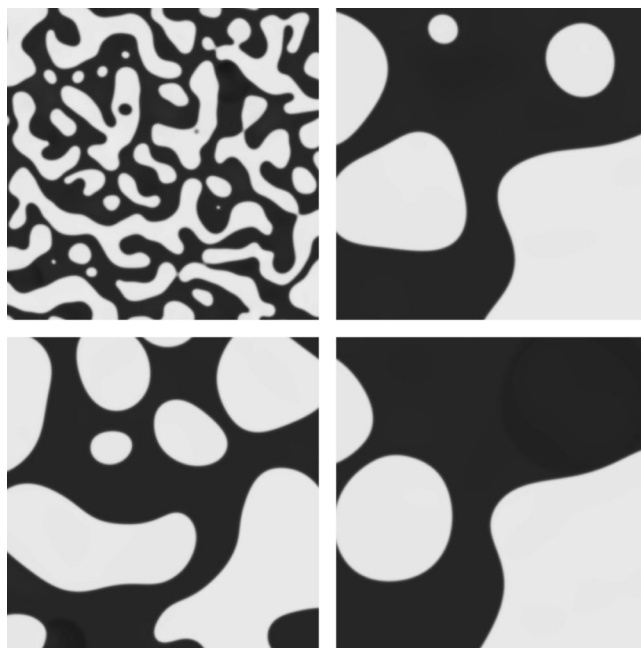
FIG. 3. Contour plots of a portion 512 \times 512 of the whole lattice of the density n in the case with \tau=10^{-4} , \beta=0.5 , and flux limiter scheme. Color code: black/white \rightarrow liquid/vapor.
