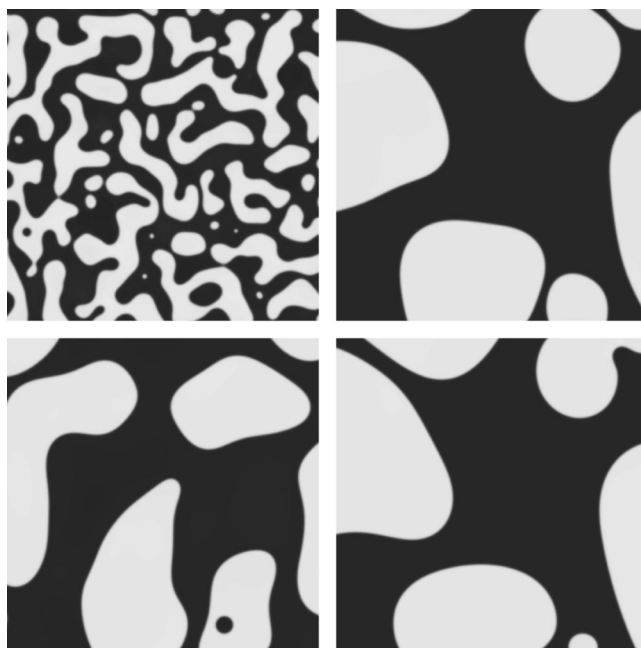
FIG. 8. Contour plots of a portion 512 \times 512 of the whole lattice of the density n in the case with \tau=10^{-3}, \beta=0.5 , and flux limiter scheme. Color code: black/white \rightarrow liquid/vapor.
